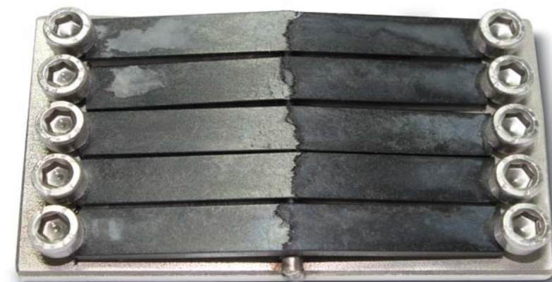
Fig. 7: Significant damage to test specimens made from standard PA6.6-GF30 after just 2 hours immersed in ZnCl 2 solution
