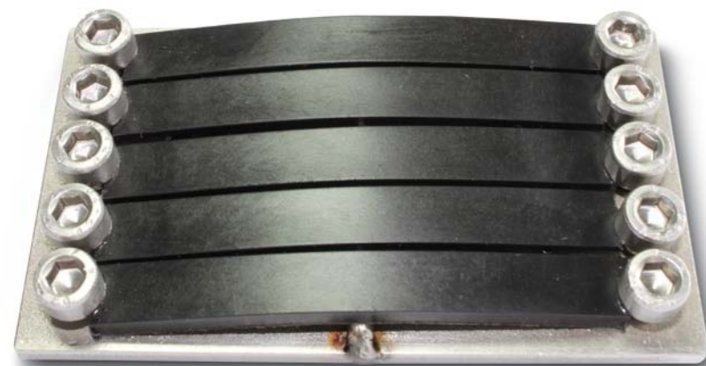
Fig. 8: No material damage of AKROMID® A3 GF 30 1 L black (4436) even after 200 hours immersed in ZnCl 2 solution
