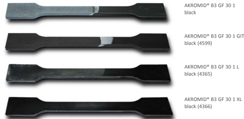
Fig. 6: Tension rods made from various AKROMID® compounds after immersion in CaCl 2 (in accordance with DBL 5416).
