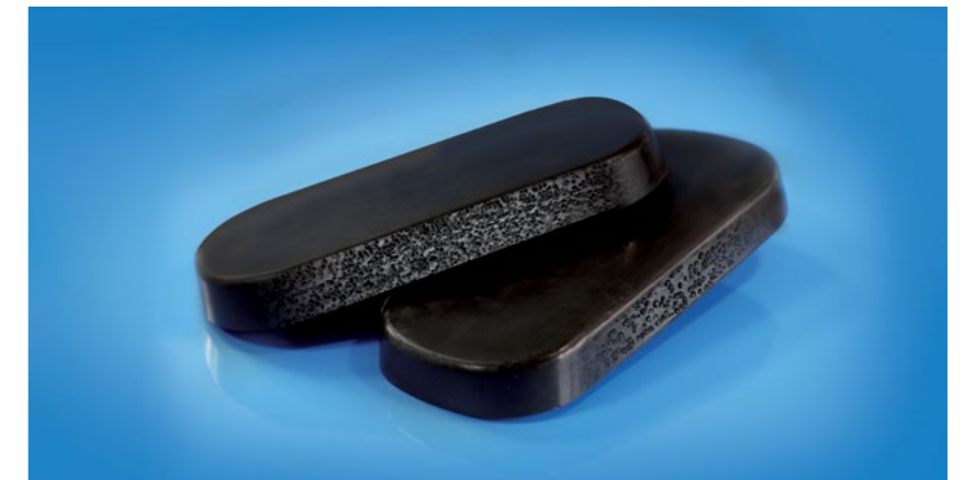
Figure 8: Foam structure with good and poor nucleation
