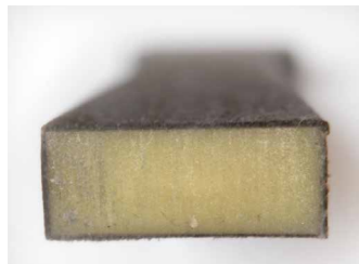
Tensile bar made of C3 GF 30 5 XTC natural (4499) after 1,000 h at 210 °C
